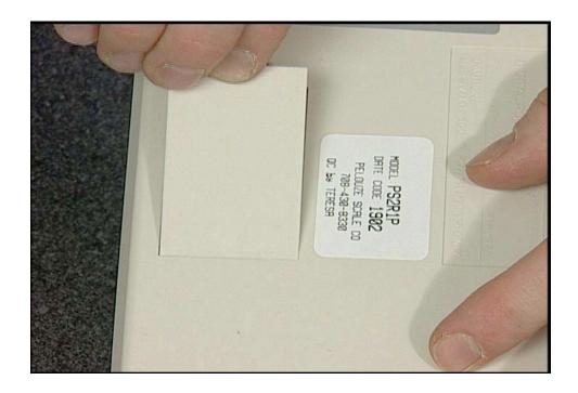
Replace the battery rate chip compartment cover.
